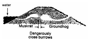
tamper. The surface of each compacted lift should be loosened to a depth of one to two inches before the next lift of material is placed. After all voids and entrances are backfilled, seed and mulch the repaired area to grow new grass and protect the slope from erosion.
